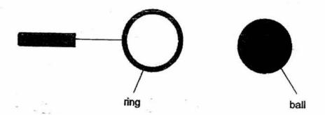
At room temperature, the ball was unable to pass through the ring. After heating the ring for a while, the ball passed through the ring.
