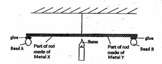
Sam heated the centre of the rod with a flame. He recorded the time taken for the bead to drop as shown in the table below.
