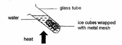
Some ice cubes were wrapped up in metal mesh to make them sink to the bottom of the tube. After a few minutes, the ice cubes have not melted completely.
